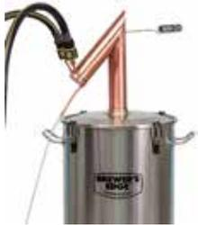
6. Now your run begins. Keep the still head cool with plenty of circulating cooling water, and collect the distillate until the still head temperature reaches 203° F. which should take about 45 minutes. When the still head reaches 203° F, the best part of the run is over, and the distillate will start to taste increasingly harsh.
