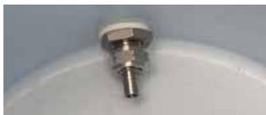
4. Now install L83 Nipple with the L86 Nut on the backside of the bulkhead The Rubbermaid cooler is shown above with its white gasket There is no need to use teflon tape.
