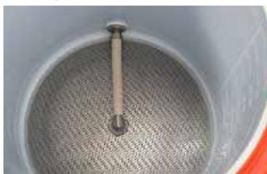
5. Finally, slip the U channel gasket over the S17 False Bottom so it covers the edge. Now place the S17 False Bottom in the cooler as shown below, and join to the bulkhead with the included Thermoplastic tubing. Rinse with water to remove manufacturing residues and you are ready to mash.
