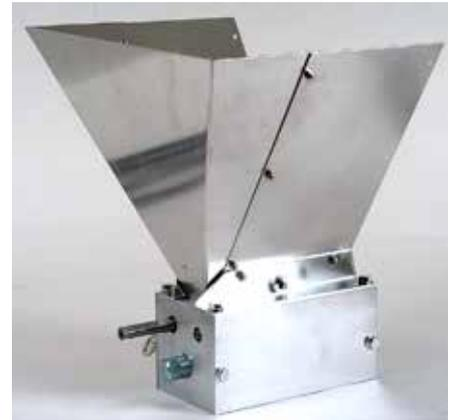
**STEP SIX:** Install the front Hopper End (part #6) with six 7mm lock nuts. Then repeat and install the back Hopper End.
