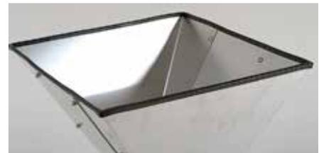
**STEP EIGHT:** Install the Rubber Hopper Finisher (part #2) by pressing into place. Now firmly tighten all 7mm locknuts and you are done with hopper assembly.
