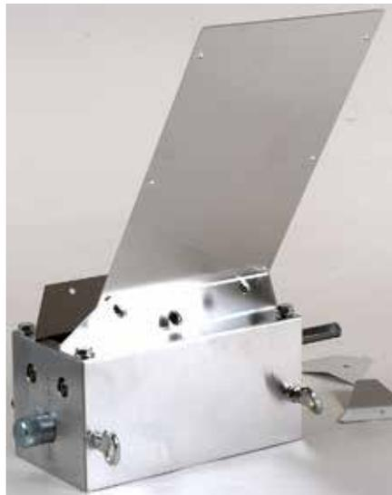
**STEP FOUR:** Attach the left side middle hopper (part #7) onto the left side of the mill with three 7mm lock nuts, using your 7mm open wrench and phillips screwdriver. Put the nuts on the outside and the screw heads on the inside for smoother grain flow. Do not over-tighten, keep all screws slightly loose at this point. Now repeat and do the other side.
