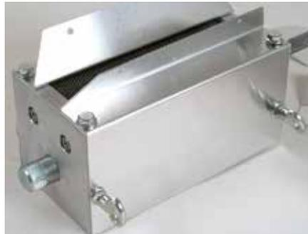
**STEP THREE:** Repeat the process for the other side of the mill, using two G88 screws and unscrewing the two adjustment thumbnuts and then reinstalling to install the Mill Body Side.
