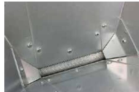
**STEP SEVEN:** Install the Hopper Anti Bind Pieces (part #4) inside both ends of the mill hopper with one 7mm locknut and phillips screw.
