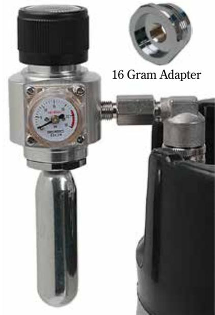
The Paramount ships with a 74 gram C02 cartridge adapter in the regulator base. To switch to 16 gram threaded cartridges, unscrew the base adapter with a large wrench, and screw in the included L15 Adapter pictured above. Be sure to include the clear washer behind the adapter to seal the C02. Tighten with a wrench and you are ready to dispense with 16 gram threaded cartridges.
