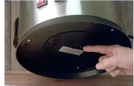
**ER4:** Thermostat overheating protection. This can happen when the heating element and thermostat are covered by a hop or grain bag. It can also be caused by heavy trub deposits resulting from too fine a grain crush, or malt extract or honey being poured into the unit, coating the thermostat. Reset by unplugging, and pressing the reset button on the bottom center of the unit.
