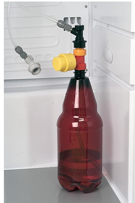
beer line faucet assembly with a standard 4' hose, you will need to pump 1/3 to 1/2 of the bottle through the line. After doing this, close the beer faucet, remove the beer line ball lock from the unit, and let the BLC Cleaner soak for 20 minutes in the line and faucet.
