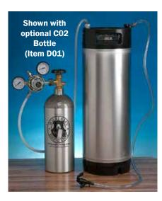
SAFETY WARNING: The C02 cylinder must be secured upright when in use. Either brace it with the keg, or fasten upright with a chain or brace (not included) to make sure it cannot fall sideways when in use. If it falls sideways when in use, liquid C02 gas could escape the regulator so fast that it would cause the keg to explode, causing personal injury.
