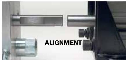
should be well enough aligned that it just slides into the mill shaft). Tighten the spider coupling, and checking alignment once more to make sure everything is straight; now drill 4 1/4" holes through the base using the already drilled motor mount holes as a guide to mount your completed motor assembly to your base board. Tighten and you are now ready to wire your mill.
