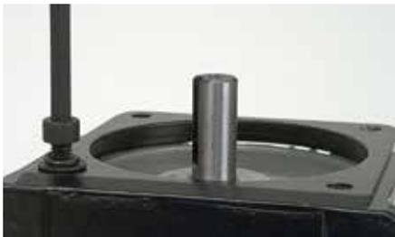
1. Install the motor mount on the motor/gear box assembly with the four 5mm hex key screws and washers so the wire comes out the top when finished. The motor can also be installed so the wire comes out on the bottom, but then you will have to shim up the Mill a 1/4" or so off the base to align with the motor shaft (we have found it is easier to shim up or down the motor than adjust the height of the mill).
