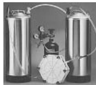
Press one stainless steel hose fitting onto the end of the outlet hose assembly, and the other on the end of the inlet hose. Screw two beer ball-lock or pin-lock keg connectors (depending on the type of kegs you have) onto the D08 stainless fittings on the hoses. Your Beer Plate Filter is now assembled and ready for use.
