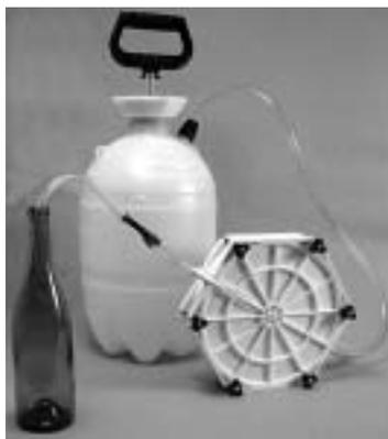
Filtering wine requires this Plate Filter, two filter pads of 3 or 1 micron rating, and a Pressure Tank (not included). Use 3 micron pads for wine that is a bit cloudy, and 1 micron pads for wine that has fallen almost clear. Just put your wine in the tank, assemble the filter and pads, and pump gently to filter.
