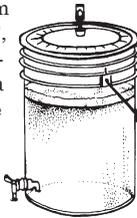
8. Sixteen days after the start of fermentation, open and check beer with a hydrometer to be sure the finishing gravity of 1.019 or less has been reached (finishing gravities vary from batch to batch, and yours may be a bit higher or lower). If the gravity is above 1.019, stir beer gently with a sanitized spoon, reseal, and wait 4 more days before rechecking.
