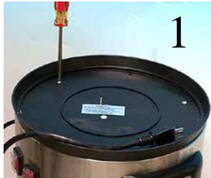
**1. UNPLUG THE UNIT.** Using a medium phillips, unscrew the three screws holding the base on. Note the position of the base and the hole for the reset switch, as you will need to replace it in the same position for the reset switch to fit through the hole. It is helpful to put some tape on the edge of the plastic bottom and another piece on the boiler to have alignment marks when you put the base back on.
