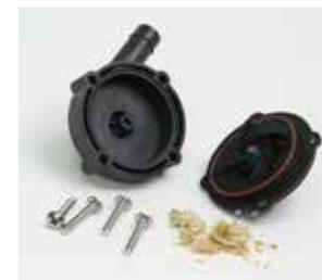
Once the head is cleaned, reassemble in the reverse order, taking care to tighten the pump head screws evenly, and slide the silicone hoses fully over the pump inlet and outlet, also sliding the nylon tie off and hose clamp so they are on securely. Replace the base and you are ready to go.
