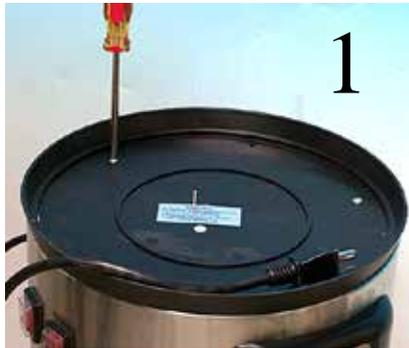
**1. UNPLUG THE UNIT.** Using using a medium phillips, unscrew the three screws holding the base on. Note the position of the base and the hole for the reset switch, as you will need to replace it in the same position for the reset switch to fit through the hole. It is helpful to put some tape on the edge of the plastic bottom and another piece on the boiler to have alignment marks when you put the base back on.
