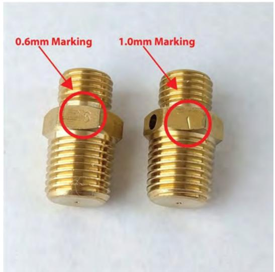
6. The different flow control devices are marked discretely with a small punch on the side of the device but if you have good eyesight you can probably see the difference in hole size with your naked eyes.
