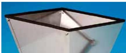
**STEP FOUR:** Now install the rubber hopper rim guard by pressing it on. Keep in mind the hopper is not square, so there is only one way it goes.
