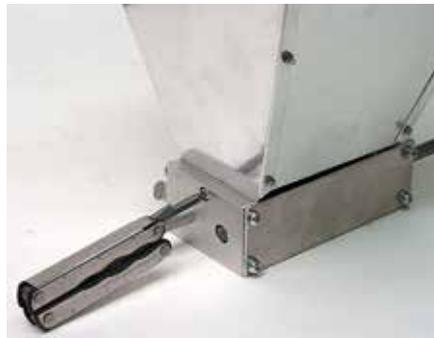
**STEP THREE:** Now attach the hopper to the mill by loosening the two center phillips hopper retaining screws and fitting the hopper lips inside the mill. This can take a little persuading and pushing, but having the hopper body screws loosened helps. Once in place, firmly tighten the two hopper retaining screws.
