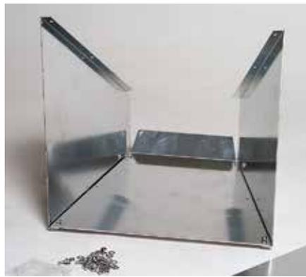
**STEP TWO:** Assemble the hopper. Use a 7/32" wrench and small phillips screwdriver. Putting the screw heads on the inside of the hopper will result in smoother grain flow. Leave all the screws a bit loose at this point.
