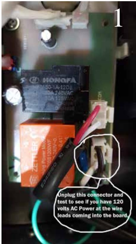
Set your multimeter to AC volts and press the leads into the connector as shown at above right. If you do not get 120 volts AC here, the power cord or plug is bad.
